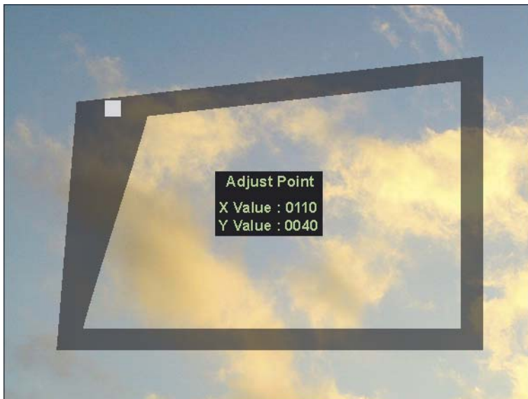
Image 2-26 Push the cursor keys ← or → to adjust the length of the vertical side
